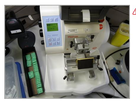
Immediately after inserting blade into microtome
